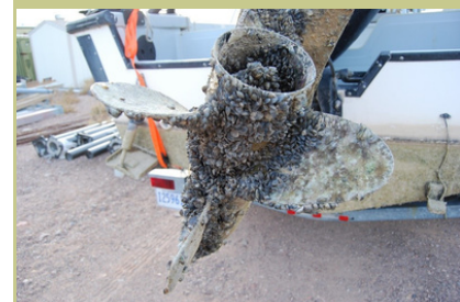
Zebra mussels coat and damage a boat motor in the Great Lakes Region.
